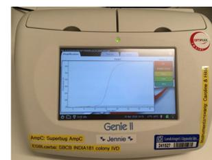
LAMP reaction and detection is monitored in real time by the GENIE II® instrument.
