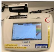
**Figure 2.** LAMP reaction and detection is monitored in real time by the GENIE®II instrument.
